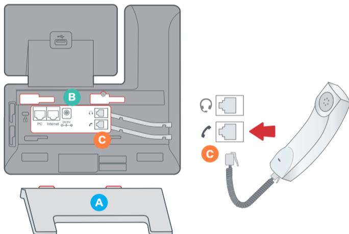
Connect the phone handset to the handset jack **C** using the coiled phone cord.
